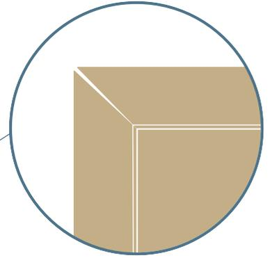
When wood swells, miter joints open as shown above.
