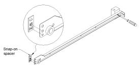
Make sure the slide is oriented as shown in the detail to the right. Snap 1/8" thick roll tray spacer onto cabinet member – as also shown in detail to the right. Repeat step for opposite cabinet member slide.
